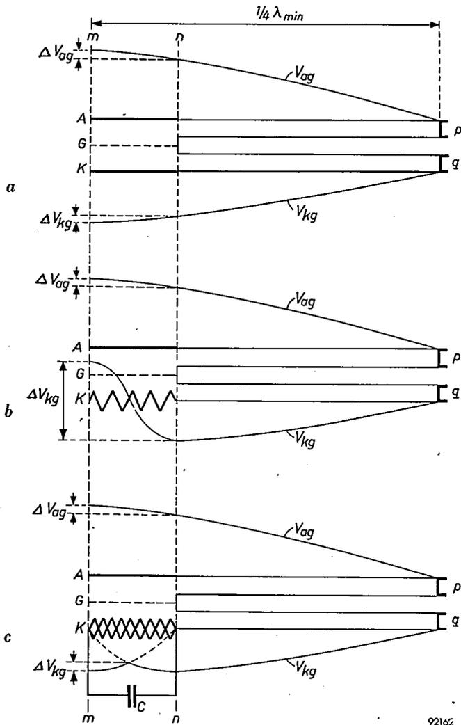
Fig. 7.  $K$  cathode,  $G$  grid and  $A$  anode of triode (schematic) showing the variation of the alternating voltages  $V_{ag}$  between anode and grid, and  $V_{kg}$  between cathode and grid, along the length of the anode and cathode respectively.  $\Delta V_{ag}$  and  $\Delta V_{kg}$  potential differences between the ends of these electrodes.  $p, q$  shorting-pistons (cf. fig. 6).  $mp = mq = \frac{1}{4}\lambda_{min}$ .
