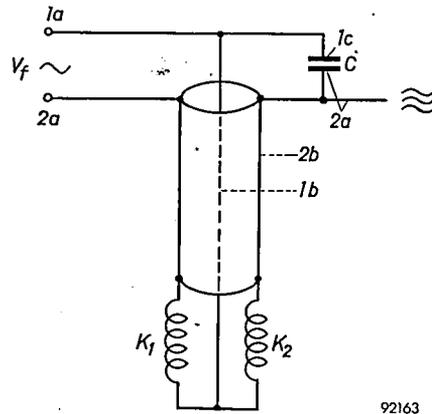
Fig. 8. The two coiled filaments  $K_1$  and  $K_2$  (shown side by side for clarity) and the capacitor  $C$ . For  $1a, 1b, 1c, 2a$  and  $2b$ , see figs. 2 and 3. The filament voltage  $V_f$  is applied between  $1a$  and  $2a$ .  $2a$  is also the connection for the high-frequency current.
