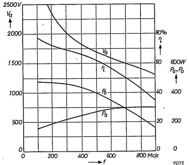
Fig. 14. Maximum permissible H.T. voltage  $V_a$ , maximum permissible dissipation  $P_a$ , power output  $P_o$  and efficiency  $\eta$  of an oscillating TBL 2/300 tube, as a function of frequency  $f$ .
