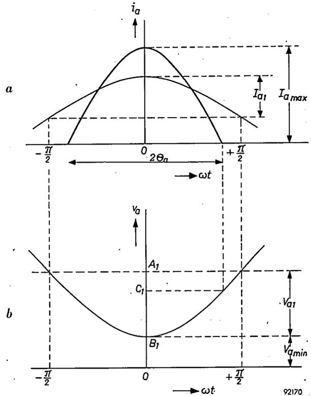
Fig. 15. a) Anode current  $i_a$ , (b) anode voltage  $v_a$  of an oscillating tube, as functions of  $\omega t$  ( $\omega = \text{angular frequency, } t = \text{time}$ ).  $2\Theta_a = \text{conduction angle}$ . Thin curve in (a): the sum of the fundamental of  $i_a$  (amplitude  $I_{a1}$ ) and the D.C. component.
