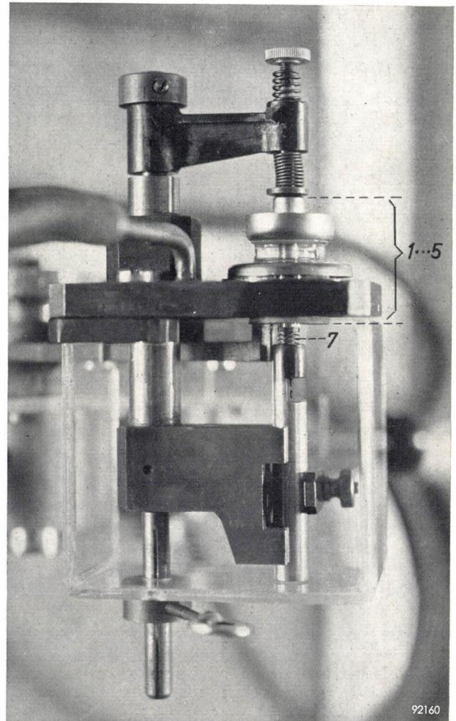
Fig. 5. The filaments *7* are brazed to the assembly *1-5* by high-frequency heating.
