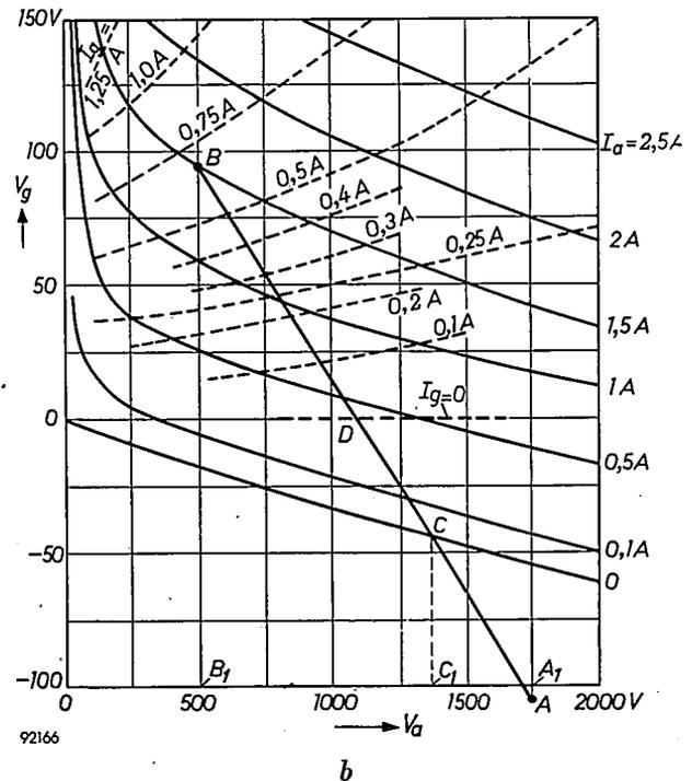
Fig. 10. Static characteristics of the TBL 2/300. a) Anode current  $I_a$  (full) and grid current  $I_g$  (dashed) as a function of anode voltage  $V_a$ , with grid voltage  $V_g$  as the running parameter. b)  $V_g$  as a function of  $V_a$  for constant  $I_a$  (full) and for constant  $I_g$  (dashed).
