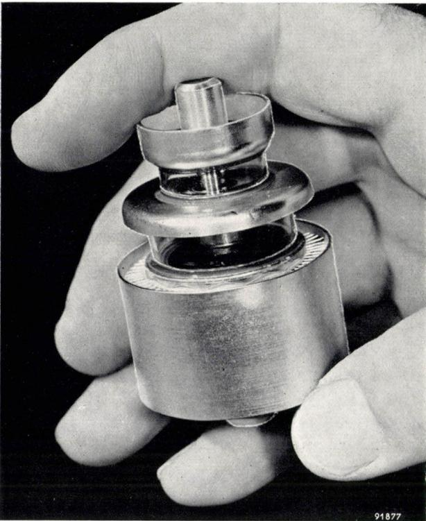
Fig. 1. The transmitting triode TBL 2/300.
